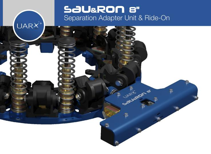
SAU&RON 8" is a reliable and efficient separation adapter for small satellites. Specially designed for those requiring a standard and dependable interface to a launch vehicle or kick stage beyond the 12U CubeSat form factor, SAU&RON 8" utilizes compression springs that can be easily configured to exert the desired separation velocity to the payload.
